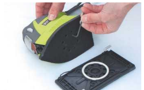
Three hex screws must be removed before the sanding base can be changed
